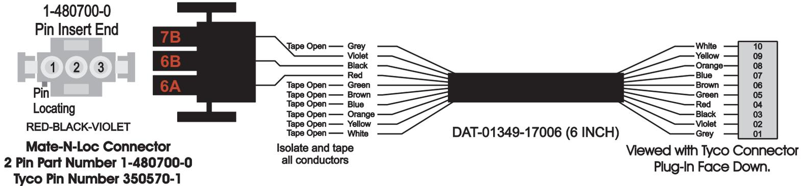
**Mate-N-Loc operates relays 6A, 6B & 7B with "IGNITION", on RCT-01760, Bus Power Center connects to J4 on RCT-01083, Dash Switch Center.**
